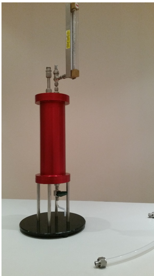
Fig.8: Condensation trap assembled with flowmeter
