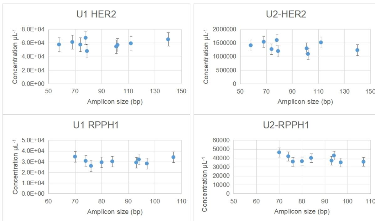
Figure 11. Participants' results as a function of amplicon size for HER2 and RPPH1 in two samples. Error bars are standard uncertainties.
