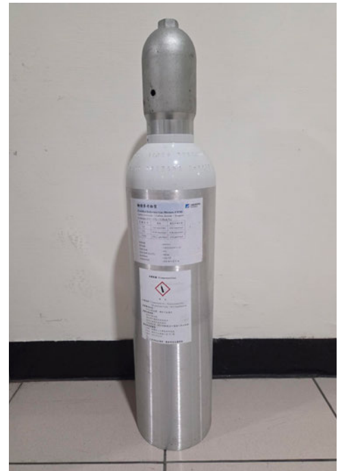
Figure 1. Reference Materials for iron oxide nanoparticles (left) and a Certified Reference Gas Mixture containing carbon monoxide, carbon dioxide, and propane in nitrogen (right).
