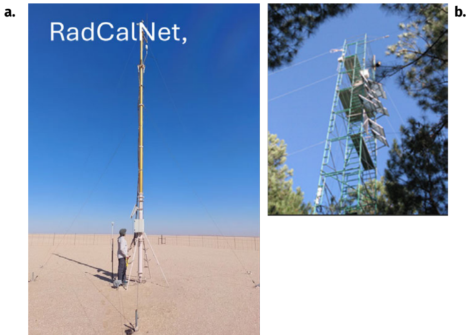
Figure 4. (Left, a) NPL managed RadCalNet tower hosting a radiometer measuring the reflectance of the Earth in the Namib desert as a reference for satellites. Right b) tower hosting NPL instruments monitoring vegetation at Wytham woods in Oxfordshire, UK.
