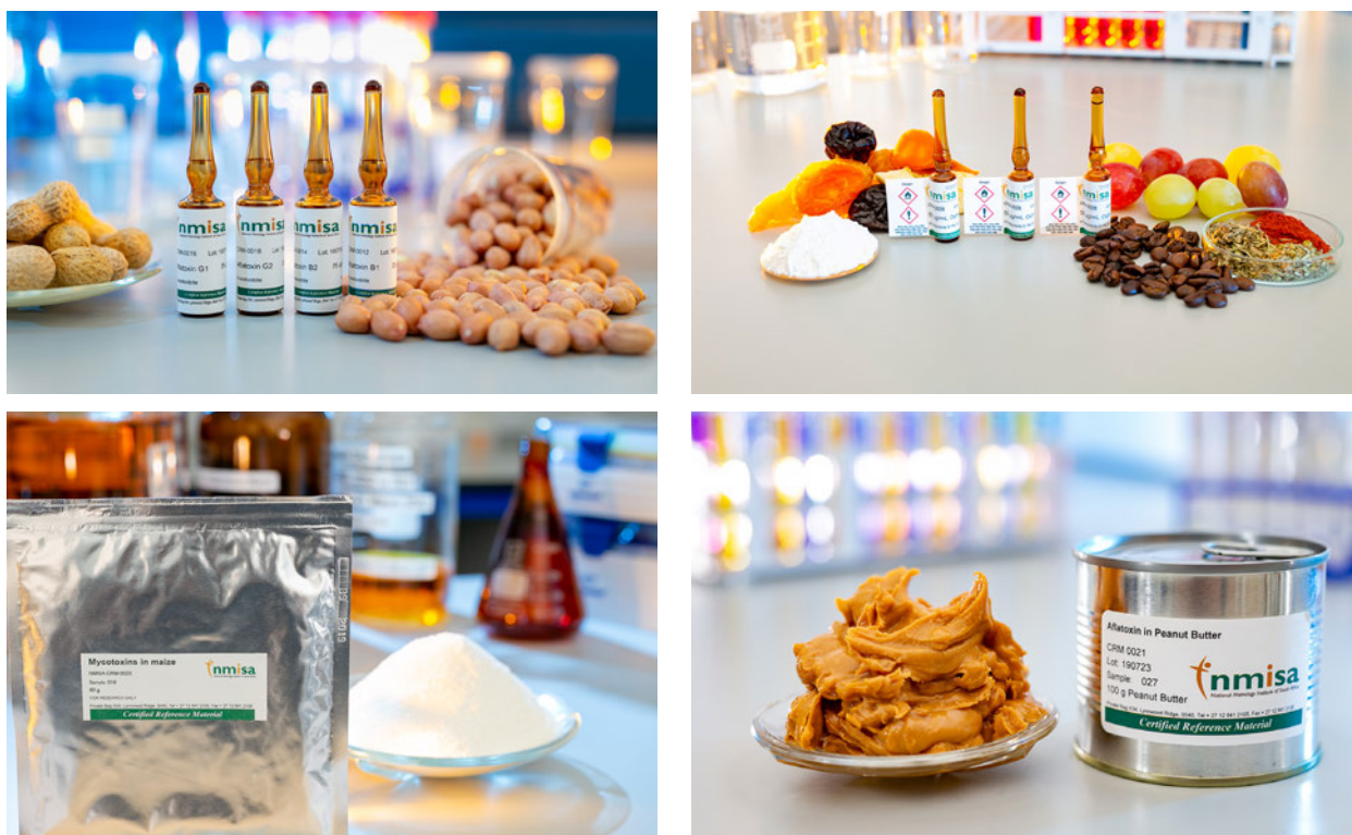
Figure 2 Clockwise: NMISA Mycotoxin calibration solution CRMs for aflatoxins B1, B2, G1, G2 (top left). NMISA Ochratoxin-A CRM solution (top right), and matrix CRMs for multiple mycotoxins in white maize (bottom left), and aflatoxins in peanut butter (bottom right). 7
