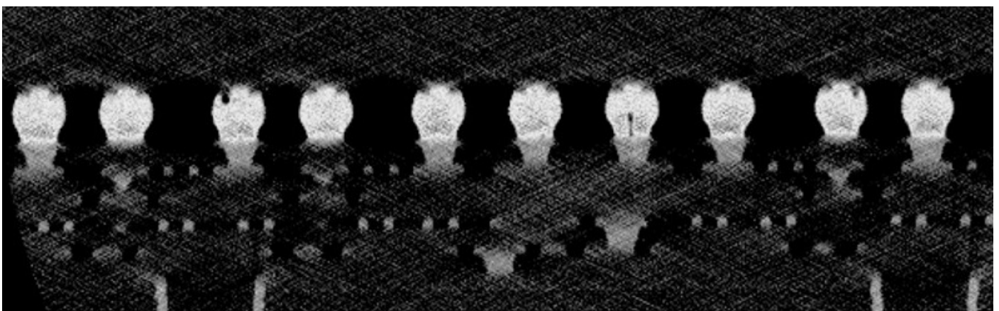
Figure 2. A typical 3D XCT image of defects and micro-bumps on silicon substrate.
