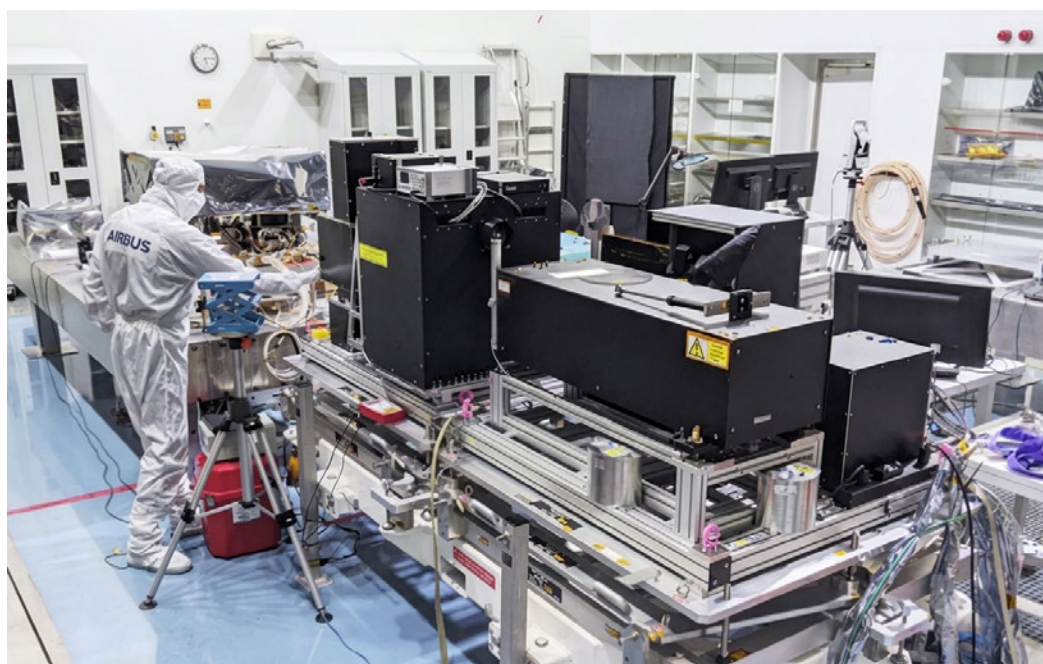
Figure 5. The NPL STAR facility shown here deployed at the Airbus cleanroom in Toulouse, France. The facility was used to calibrate the French/UK MicroCARB mission for GHG monitoring.
