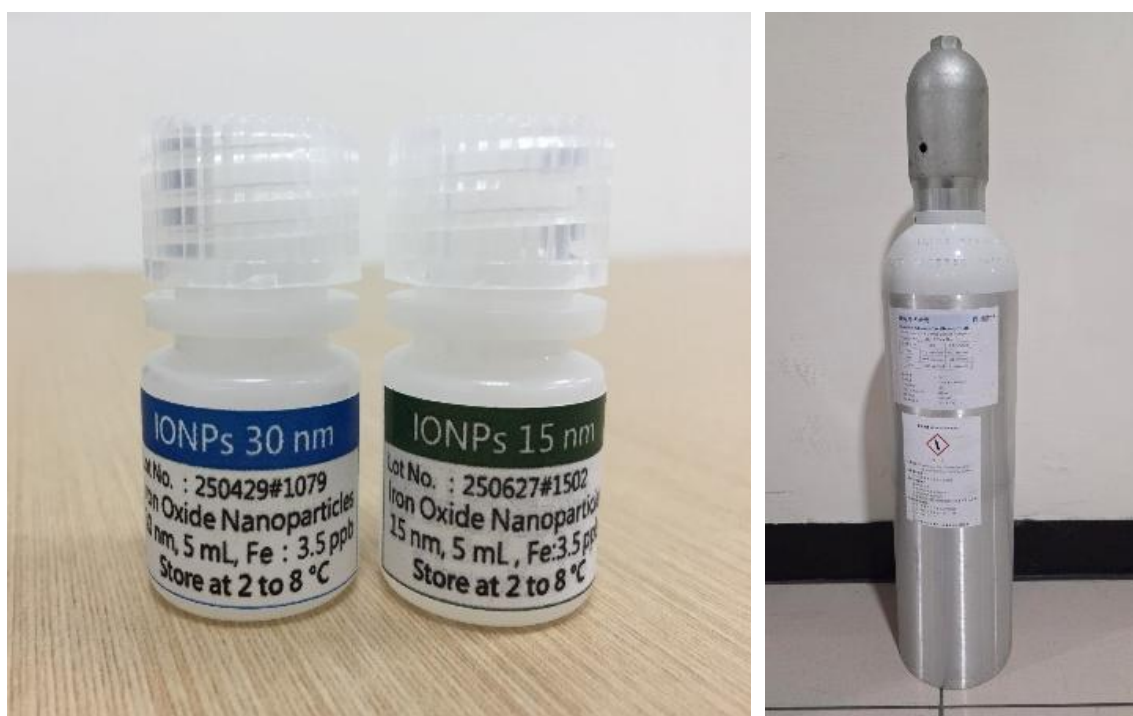
Figure 1. Reference Materials for iron oxide nanoparticles (left) and a Certified Reference Gas Mixture containing carbon monoxide, carbon dioxide, and propane in nitrogen (right).
