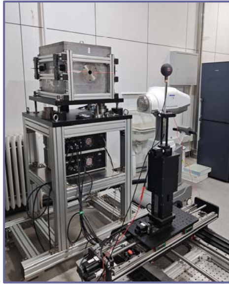
Figure 1. Set-up for the calibration of HDR brachytherapy source at the NIM
