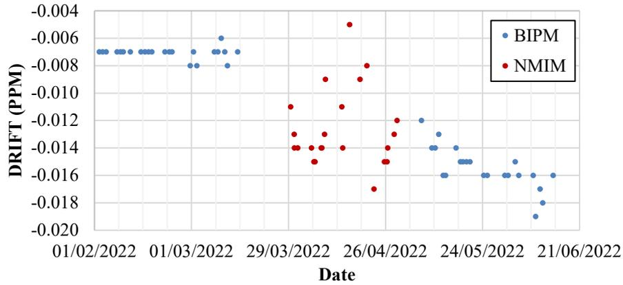
Figure 5 “DRIFT (PPM)” front panel readings of the 10 pF capacitor SN 02280.
