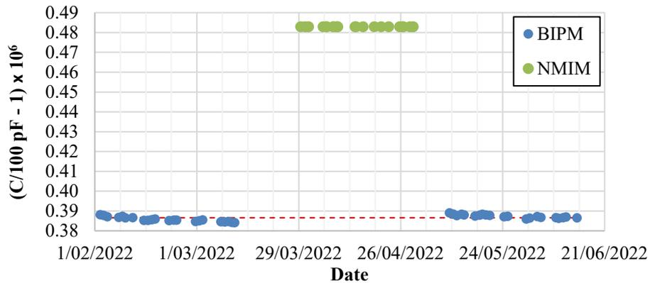
Figure 6 BIPM and NMIM measurements for the 100 pF capacitor SN 01574 at 10 V (rms) and 1000 Hz.
