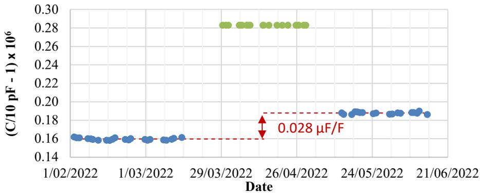
**Figure 8 BIPM and NMIM measurements for the 100 pF capacitor SN 02188 at 10 V (rms) and 1000 Hz.**
