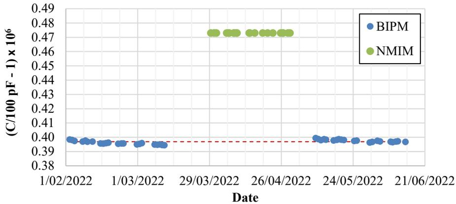
**Figure 7 BIPM and NMIM measurements for the 100 pF capacitor SN 01574 at 10 V (rms) and 1592 Hz.**
