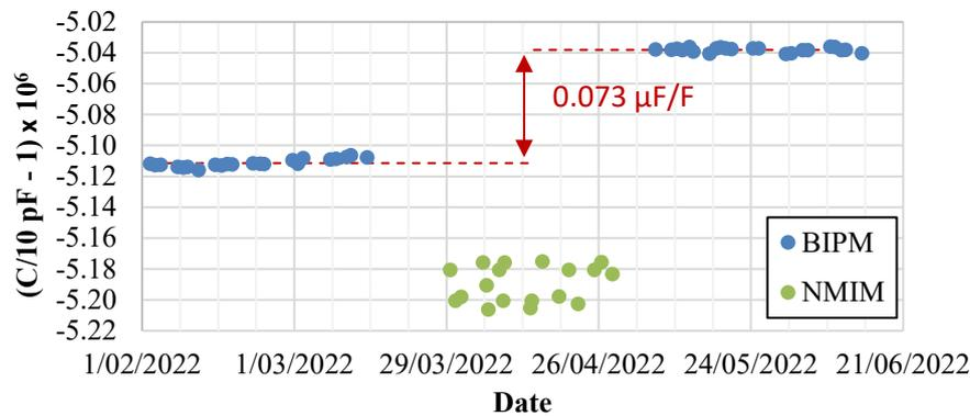
Figure 1 BIPM and NMIM measurements for the 10 pF capacitor SN 02213 at 15 V (rms) and 1000 Hz.
