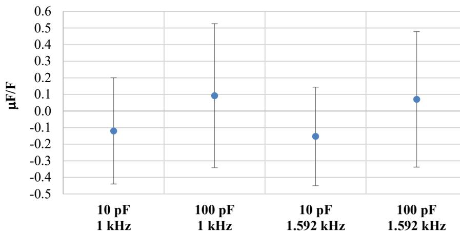
**Figure 11 Degree of equivalence between the BIPM and the NMIM for 10 pF and 100 pF capacitance measurements and associated uncertainty ( $k = 2$ ).**
