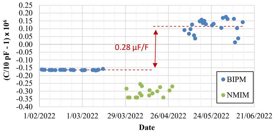
**Figure 3 BIPM and NMIM measurements for the 10 pF capacitor SN 02280 at 15 V (rms) and 1000 Hz.**
