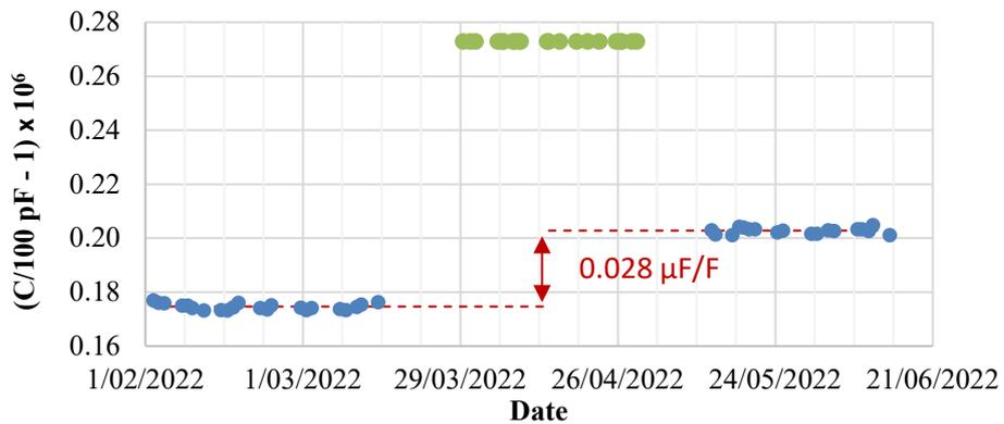
**Figure 9 BIPM and NMIM measurements for the 100 pF capacitor SN 02188 at 10 V (rms) and 1592 Hz.**
