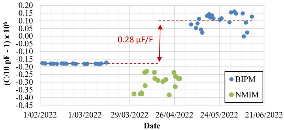
**Figure 4 BIPM and NMIM measurements for the 10 pF capacitor SN 02280 at 15 V (rms) and 1592 Hz.**
