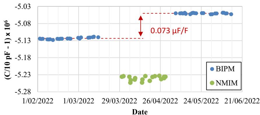
Figure 2 BIPM and NMIM measurements for the 10 pF capacitor SN 02213 at 15 V (rms) and 1592 Hz.
