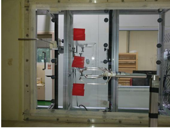
Figure 1 TS is calibrated by the Pitot tube in KRISS wind tunnel
