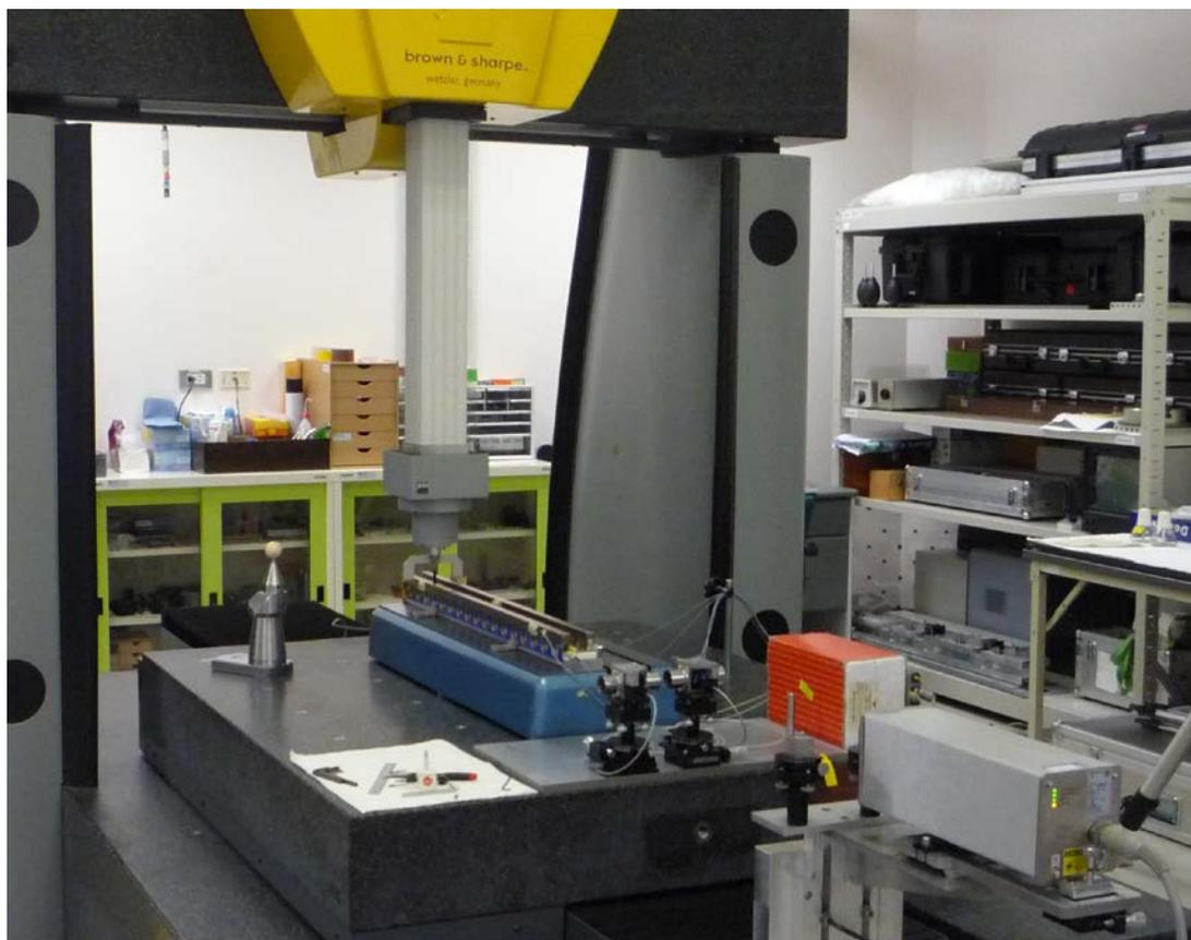
Figure 3. Photo shows an overview of the step gauge measurement.
