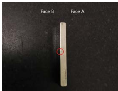
Figure 5 - Photo (provided by NMIM) of the 3 mm steel gauge block showing a dent on the edge of face B.
