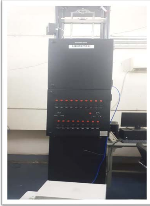
Recently established 5 kN Force Primary Standard BMC \pm 0.008 (at k=2 )
