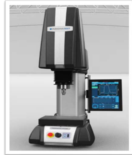
Rockwell Hardness machine to be established soon BMC \pm 0.3/\pm 0.5 HR \pm 0.4/\pm 0.6 HRN/T (at k = 2 )
