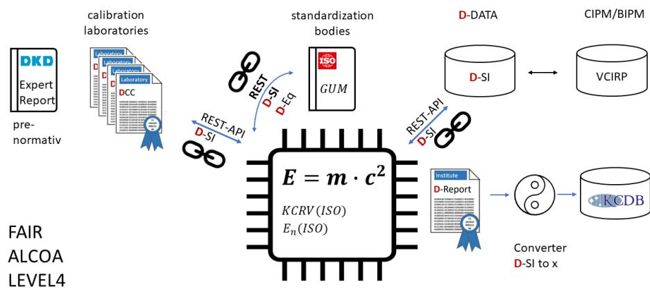
The illustration shows the interaction of a digital metrological twin (**D-TM**), shown here as a processor. This communicates via a digital interface (REST API) with data sources and machine-interpretable standards. A result report is output. The implementation also took into account developments that were decided at the last CGPM meeting and at the CIPM meeting.
