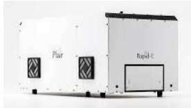
Rapid-E (Plair, Switzerland) Elastic light scattering UV-LIF Machine learning
