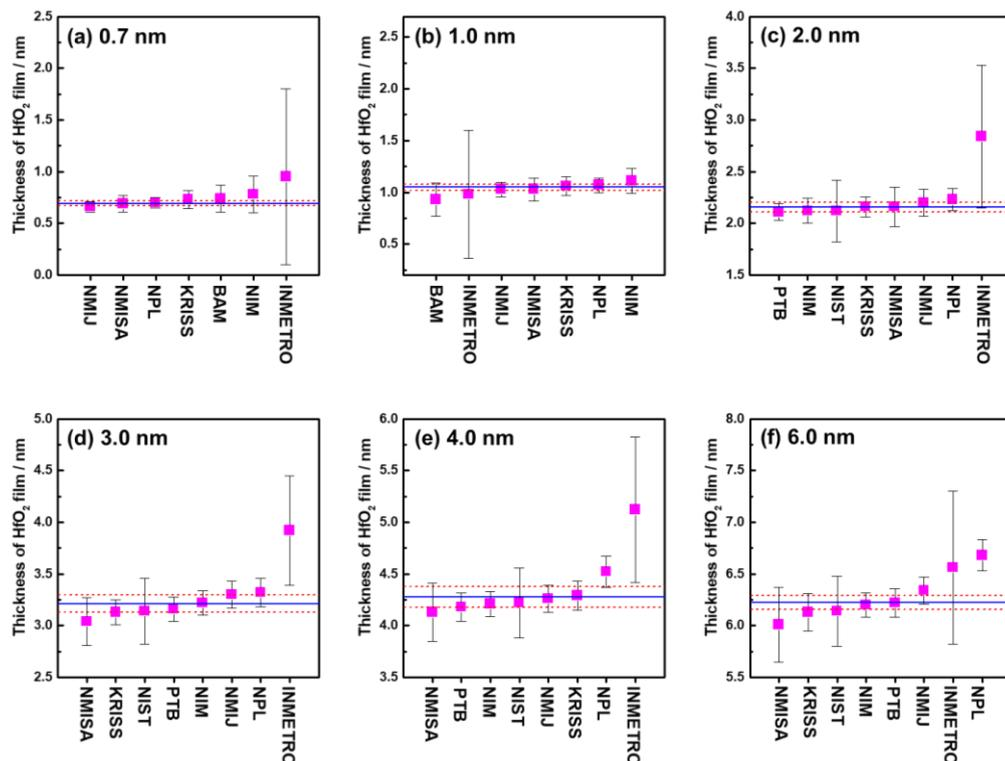
Figure 1. Key comparison reference values and their uncertainties in CCQM-K157 for six HfO<sub>2</sub> films. The solid blue lines and the broken red lines are the key comparison reference values and their standard uncertainties.
