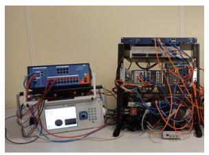
reference SAMU. Within the current Digital-IT project, that started in 2021, the bandwith of the setup will be improved enabeling characterization of SAMUs following the IEC 61869-13.
