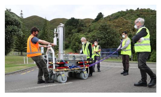
Carefully transporting the delicate MSL Calculable Capacitor to the new laboratory. Jacks on the trolley are used to keep the capacitor level at all times. Loading and offloading the capacitor together with the move took around three days.
