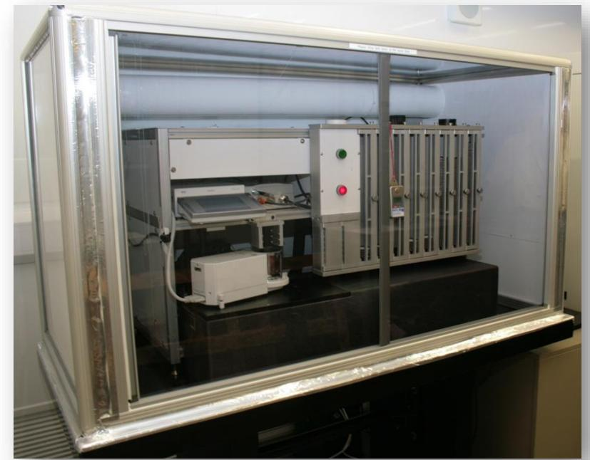
Conditioning and automatic weighing facility to weigh filters to the requirements of EN 12341:  $(47 \pm 2.5) \% \text{ RH}$ ,  $(20 \pm 1) ^\circ\text{C}$  for  $\text{PM}_{2.5}$  and  $\text{PM}_{10}$
