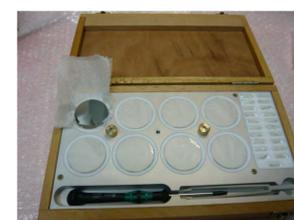
1 kg stack of 8 Pt-Ir disks fabricated at the BIPM
