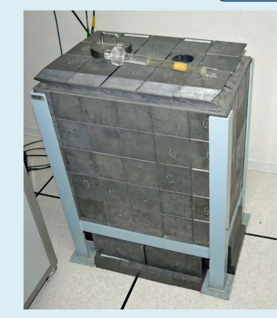
SIR = comparator based on **pressurized ionization chambers** maintained at the BIPM since 1976.
