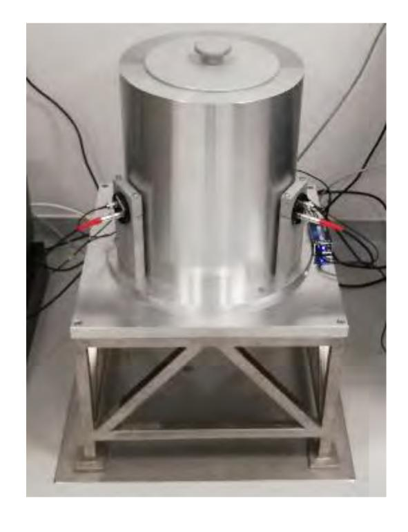
ESIR = comparator based on liquid scintillation counting, able to measure pure \(\beta\)-emitters not suited for the SIR
