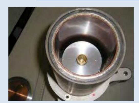
SIRTI = comparator based on NaI(TI) scintillator, linked to the SIR and travelling to NMIs.
