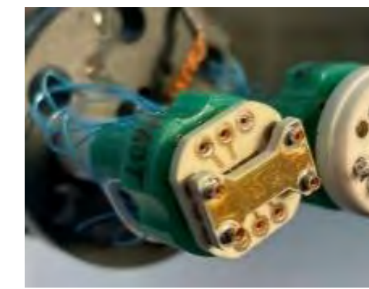
graphene QHR sample, developed by PTB
