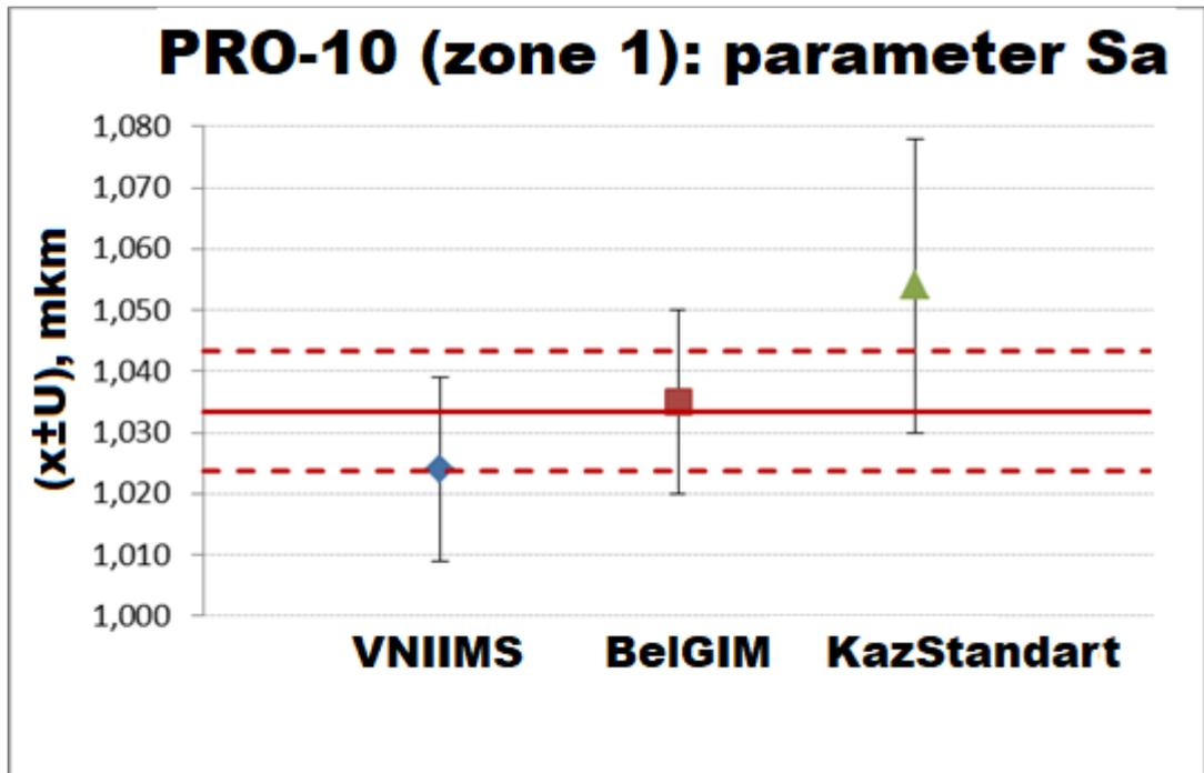
Figure 5 – Measured value of the Sa parameter in zone 1 PRO-10 (the red solid line is the reference value; the red dashed line is the extended uncertainty of the reference value)
