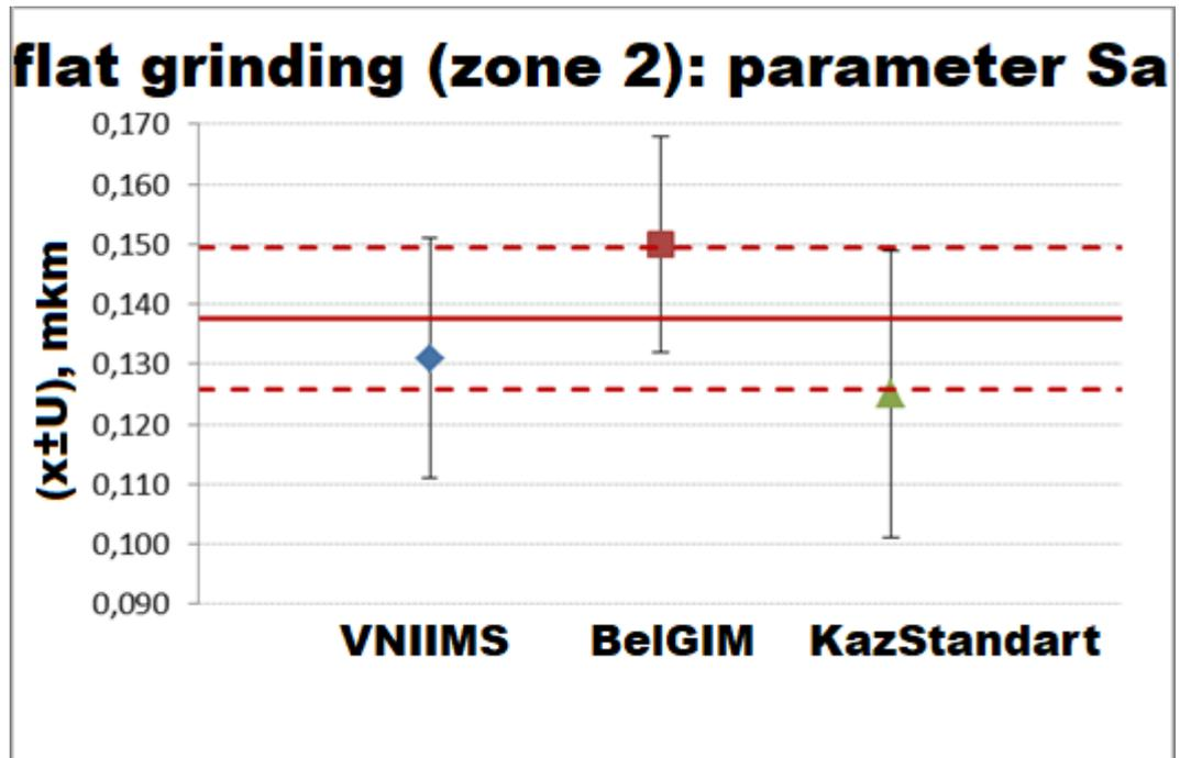
Figure 7 – Measured value of the parameter Sa in zone 2 flat grinding (the red solid line is the reference value; the red dashed line is the extended uncertainty of the reference value)
