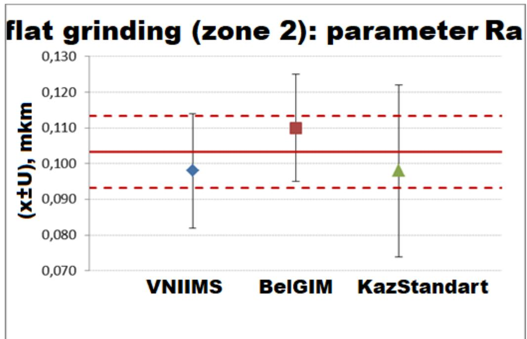
Figure 8 – Measured value of the parameter Ra in zone 2 flat grinding (the red solid line is the reference value; the red dashed line is the extended uncertainty of the reference value)
