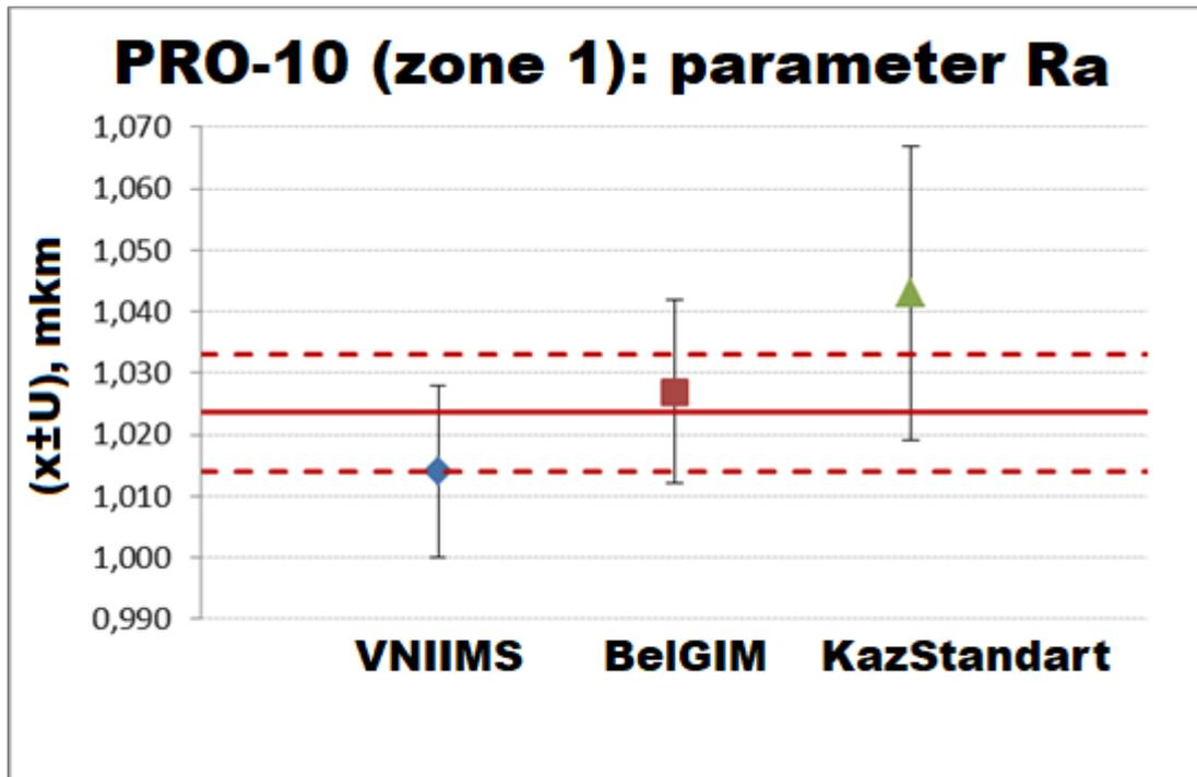
Figure 6 – Measured value of the parameter Ra in zone 1 PRO-10 (the red solid line is the reference value; the red dashed line is the extended uncertainty of the reference value)
