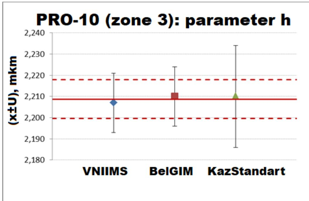
Figure 9 – Measured value of the groove depth in zone 3 PRO-10 (the red solid line is the reference value; the red dashed line is the extended uncertainty of the reference value)
