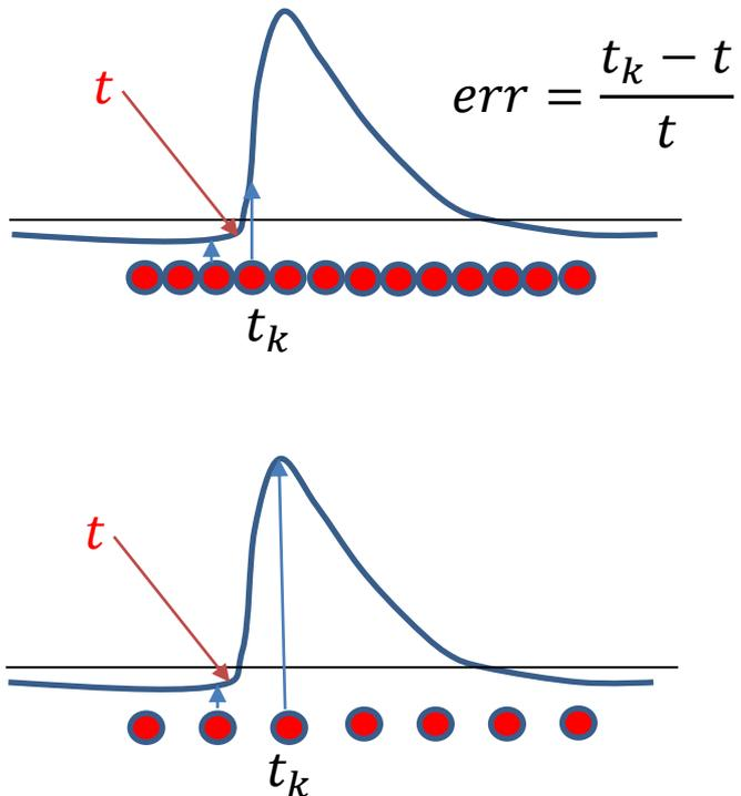
Monte-Carlo estimation of the live-time measurement error for different input count rates
