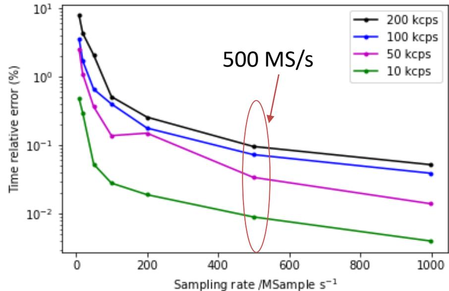
$$err(liveTime) = n^{-1} \sum_{i=1}^n \frac{t_k^{(i)} - t^{(i)}}{\Delta t^{(i)}} \text{ with } \Delta t^{(i)} \sim \varepsilon(R^{-1})$$
