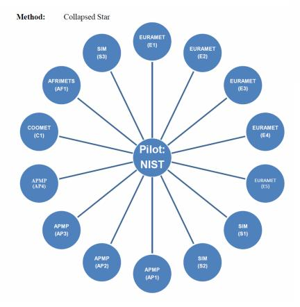
**Objective:** This comparison is designed to compare the realization of the ITS-90 through the calibration of SPRTs. The range of temperature covered in this comparison is from the triple point of Ar (83.8058 K) to the freezing point of Zn (692.677 K). The transfer standards used will be long-stem SPRTs.
