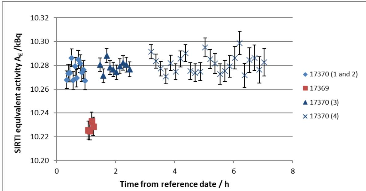
Figure 2a: Preliminary  $^{18}\text{F}$  measurement results in the SIRTl at the NRC. The uncertainty of the  $^{18}\text{F}$  activity concentration, which is constant over all the measurements, is not included in the uncertainty bars shown on the graph.
