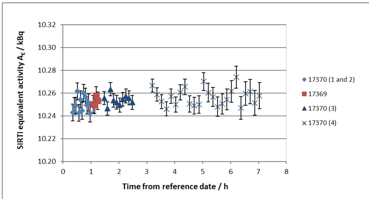
Figure 2b: Final  $^{18}\text{F}$  measurement results in the SIRTl at the NRC. The uncertainty of the  $^{18}\text{F}$  activity concentration, which is constant over all the measurements, is not included in the uncertainty bars shown on the graph.
