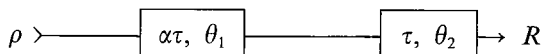
Fig. 6.2. — Schematic arrangement of two generalized dead times ( \tau, \theta ) and the relevant count rates. The input is assumed to be Poissonian.
