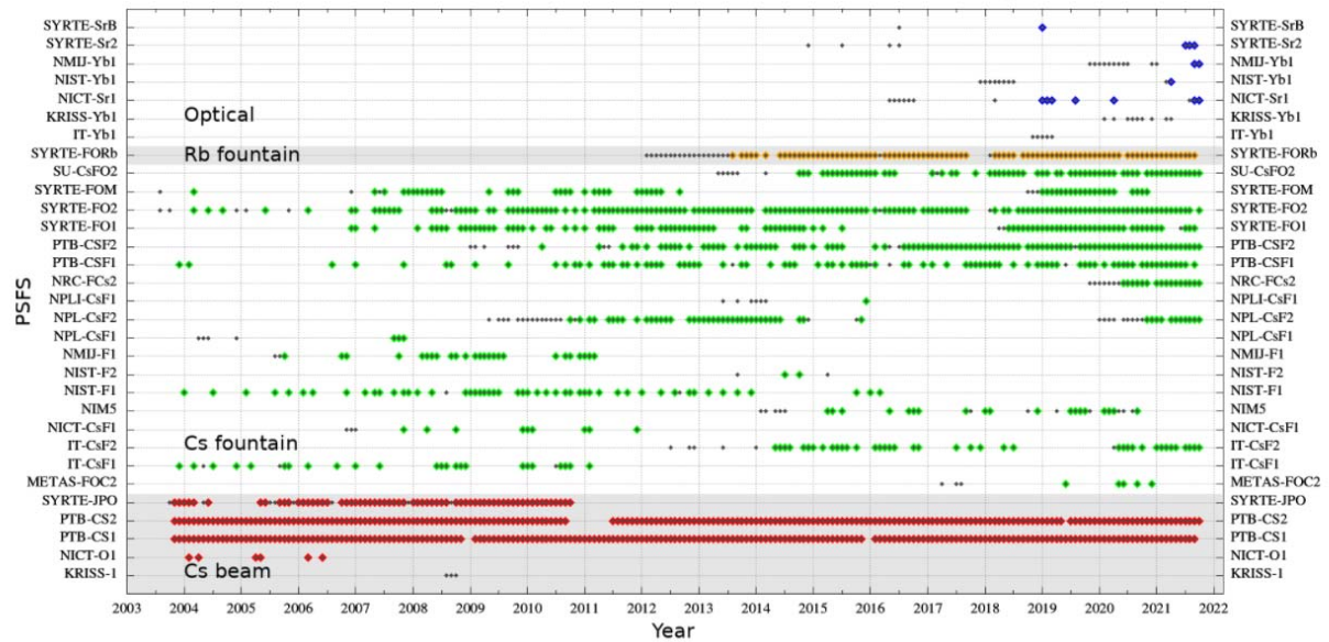
Graphical representation of all evaluations of Primary and Secondary Frequency Standards reported since Circular T 190. Enhanced color dots indicate evaluations carried out within the month of TAI computation.
