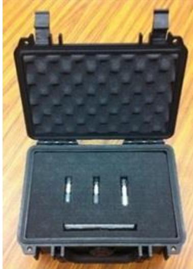
Figure 4: Shipping container with three indenters
