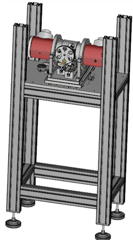
**Figure 1.** Design of the new x-ray tube support showing the automated filter wheel.
