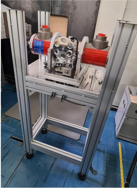
*Figure 2. Photograph of the new x-ray tube support in its temporary location.*
