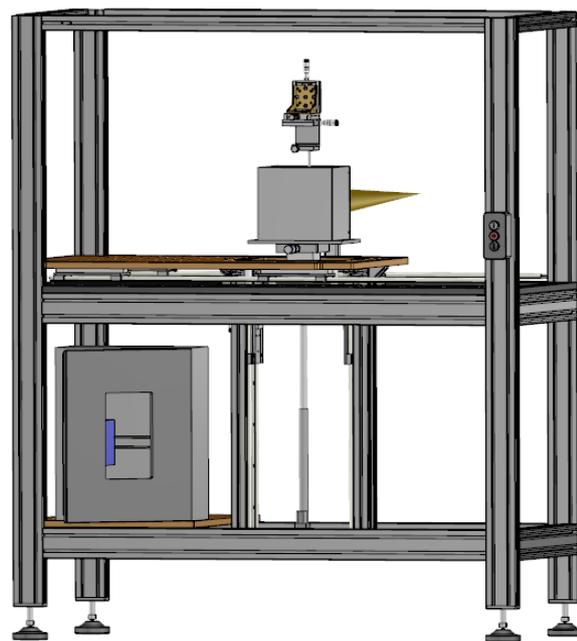
*Figure 3. Design of the new measurement bench showing the water phantom in its raised position with the cavity chamber support above it.*
