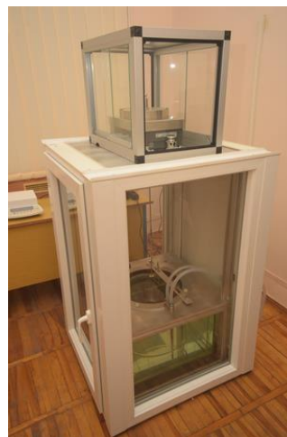
Installation of hydrostatic weighing for determining the volume of weights
