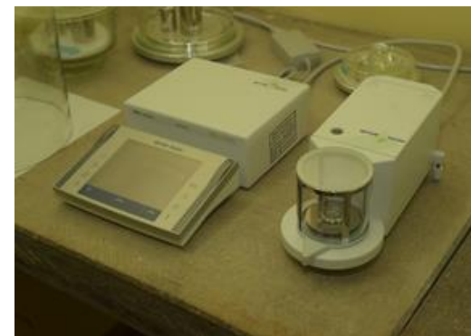
Mass comparator for mg range
