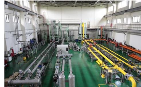
Water Flow and Oil Flow Calibration System
