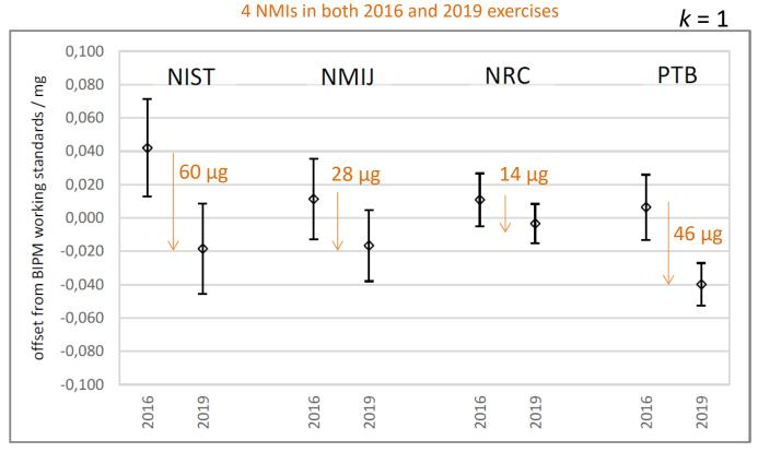
Realization experiments have changed wrt BIPM as-maintained mass unit by -14  $\mu g$  to -60  $\mu g$
