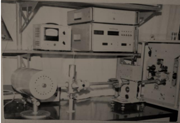
Highly sensitive measuring complex for measuring plasma parameters
