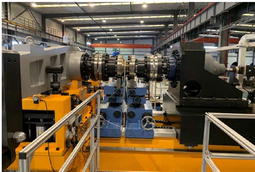
Fig. 3 100 kN•m torque standard machine
