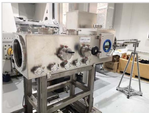
Fig. 2 The vacuum transfer equipment with Joule balance
