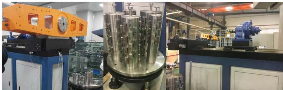
Fig. 4 The 1 kN·m torque standard machine
