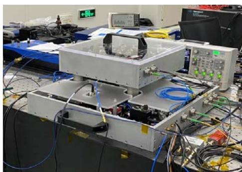
Fig.7 Raman laser system of NIM-AGRb-2.
