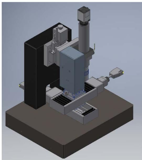
Fig.5 Hardware structure of Martens hardness tester
