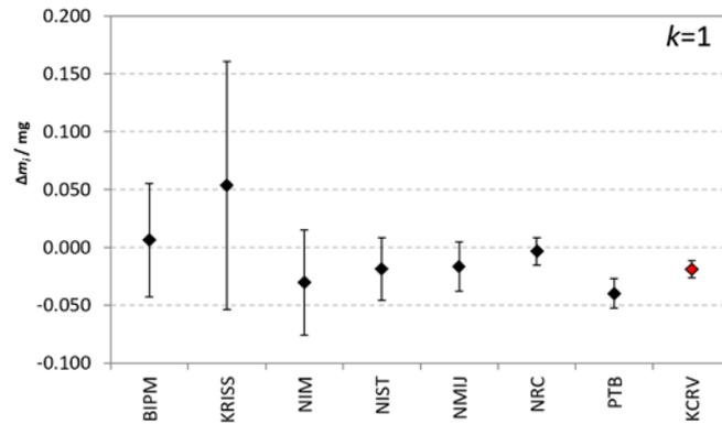
Fig. 1: the final comparison result of the CCM.M-K8.2019
