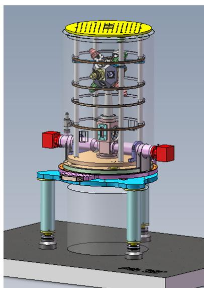
Fig.6 The physical package of NIM-AGRb-2.
