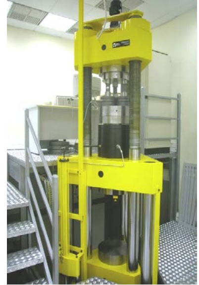
Fig. 7. Built-up type force standard machine
