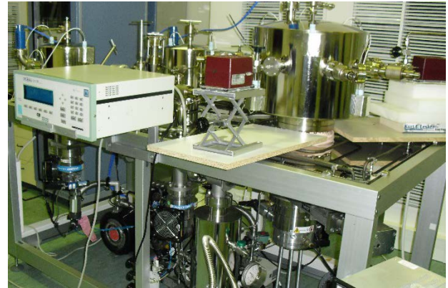
Fig.14. Primary Vacuum Static Expansion System designed and constructed by TÜBİTAK UME
