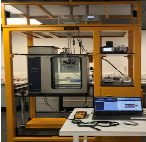
Fig. 1. Primary level hydrostatic weighing system for density determinations designed and developed at TÜBİTAK UME
