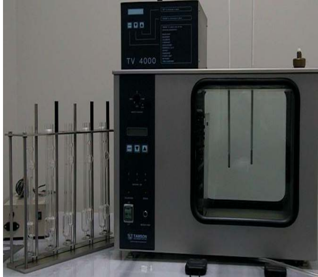
Fig. 2. Primary level viscosity measuring system
