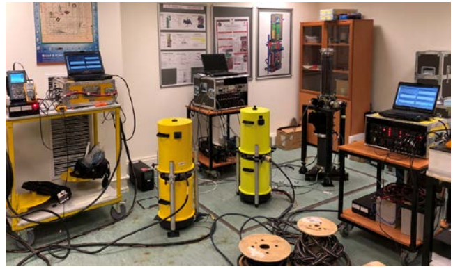
Fig. 9b. Absolute gravimeters A10 and FG5-X
