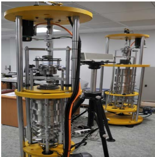
Fig.10. Rockwell, Brinell and Vickers scale deadweight hardness standards designed and constructed by TÜBİTAK UME
