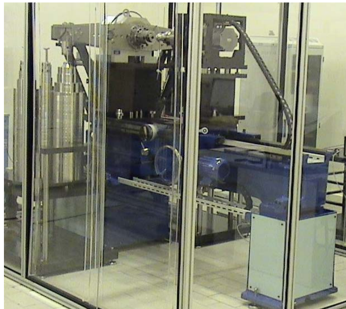
Fig. 8. 1 kN·m torque standard machine designed and constructed by TÜBİTAK UME
