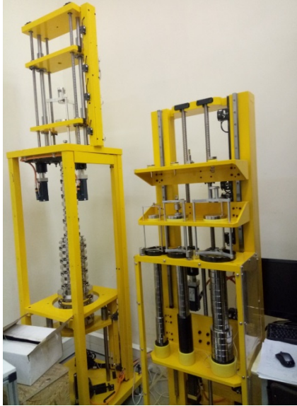
Fig. 5. Deadweight Force standard machine designed and constructed by TÜBİTAK UME
