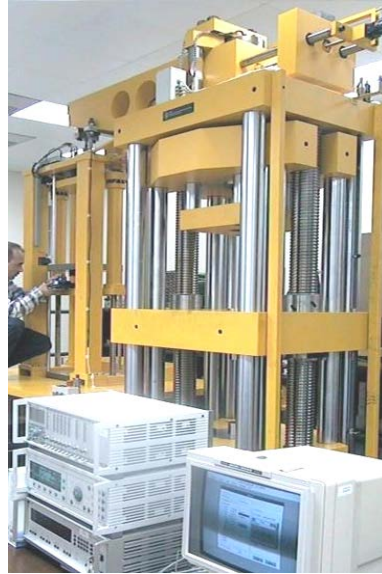
Fig. 6. Lever Amplification Deadweight Force standard machine
