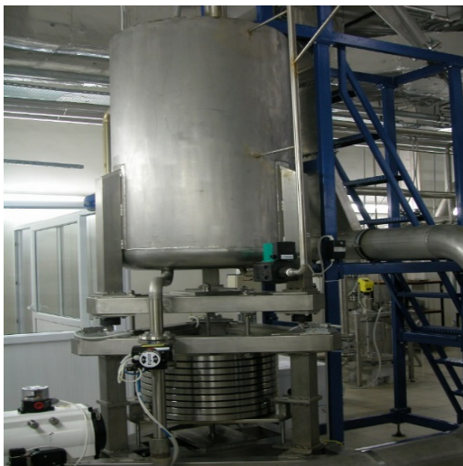
Fig. 3. 1-ton mass water flow measuring system with deadweight test mechanism
