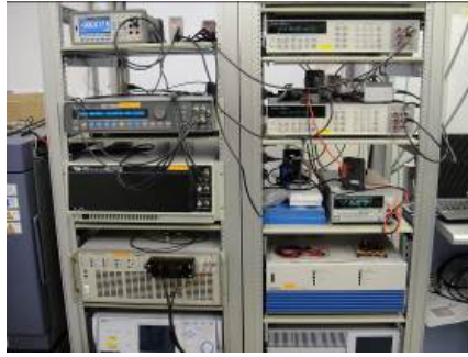
Fig. 4 Photograph of the electrochemical impedance measurement system developed using the Frequency Response Analyzer and the Potentio-Galvano Stat.
