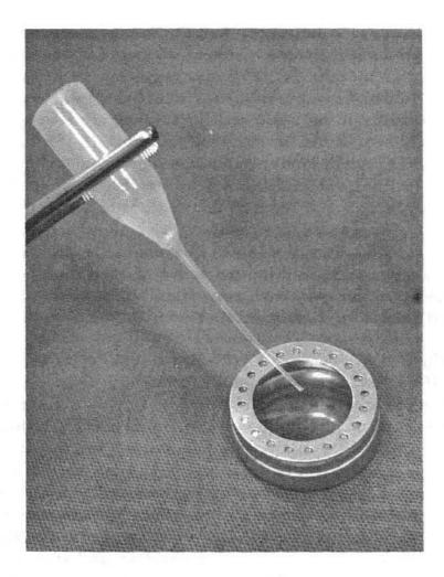
Figure 4 - Tweezers for handling pycnometers (from reference [16])
