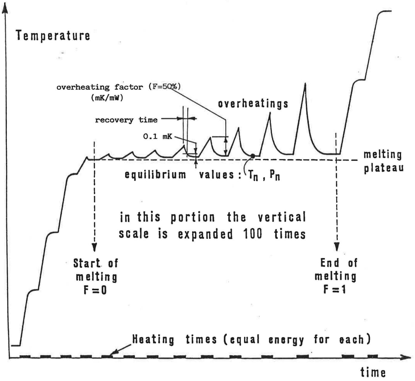
Fig.VII.3: Definitions of overheating factor and recovery time.
