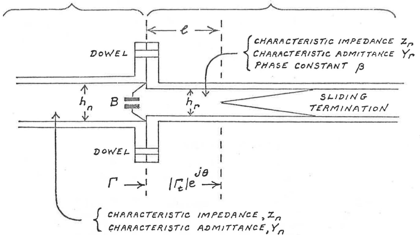
FIGURE 5. TRAVELLING STANDARD CONNECTED TO REFERENCE WAVEGUIDE ON MEASUREMENT SYSTEM
