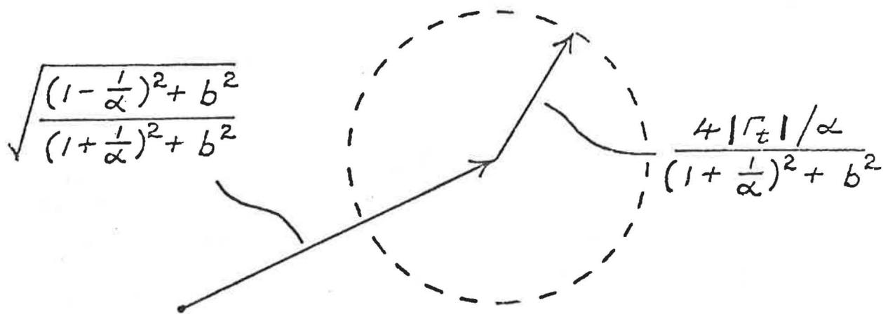
FIGURE 7. VECTOR DIAGRAM SHOWING THE TWO SIGNIFICANT COMPONENTS OF THE REFLECTION COEFFICIENT.
