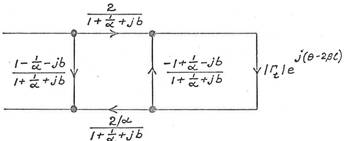
FIGURE 6. SIGNAL FLOW GRAPH FOR STEP AND SLIDING TERMINATION
