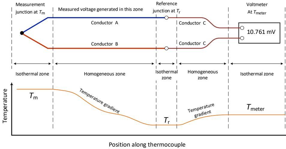
**Figure 2.** Simple thermocouple circuit and the temperature profile along it. Ideally, each part of the thermocouple exposed to a temperature gradient and generating the voltage is homogeneous, and every part where there may be inhomogeneities is isothermal.
