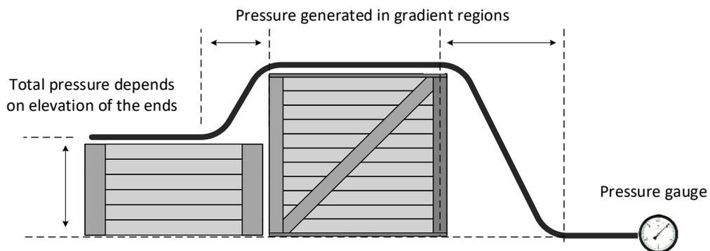
**Figure 1.** Hydraulic analogue of the Seebeck effect. Pressure differences in a fluid-filled tube are generated at gradients, but the total pressure generated depends only on the difference in the elevation of the ends of the tube.
