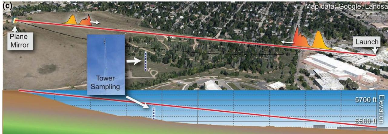
Broadband spectroscopy of several thousand molecular absorption features recorded simultaneously
