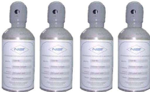
For a gas mixture, the mole fraction ( $\chi$ ) is provided by a gravimetric gas standard
