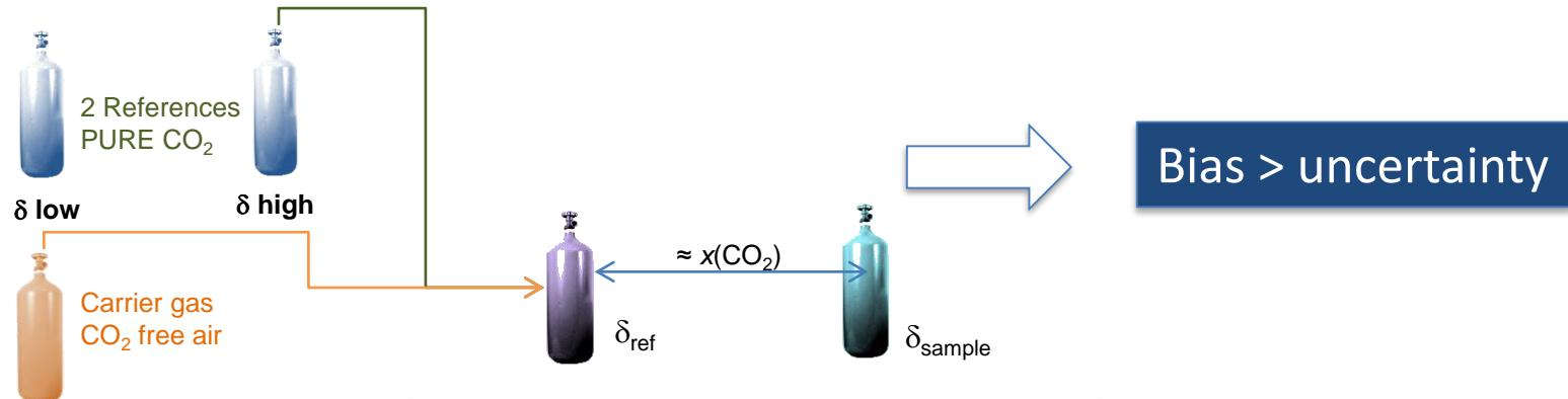
Modified calibration : add 2 CO<sub>2</sub> in air references and perform a 2 point calibration of δ values
