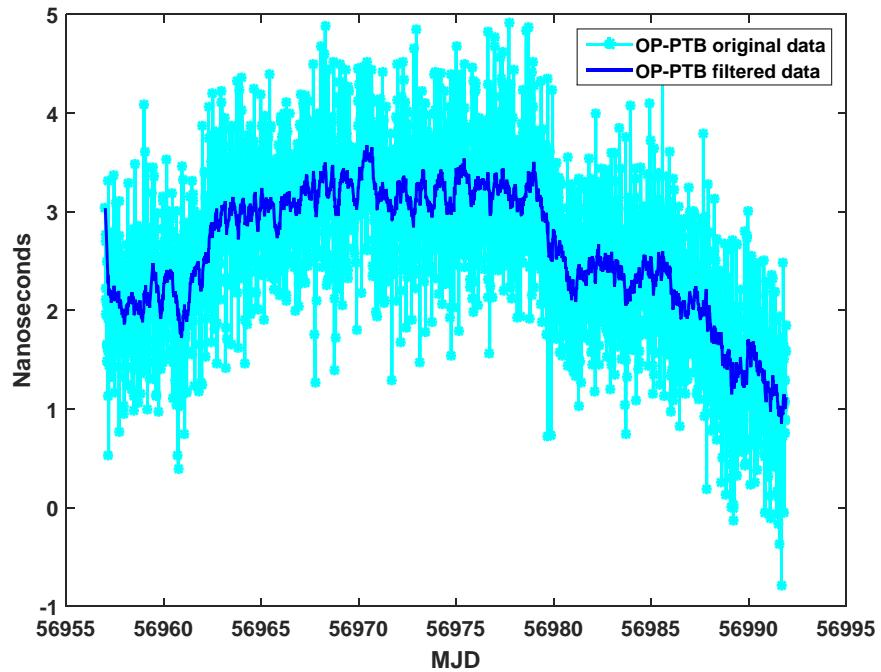
The Kalman Filter routine is used principally as a filter to noisy measurements to clean white noise (characteristic of time transfer noise).
