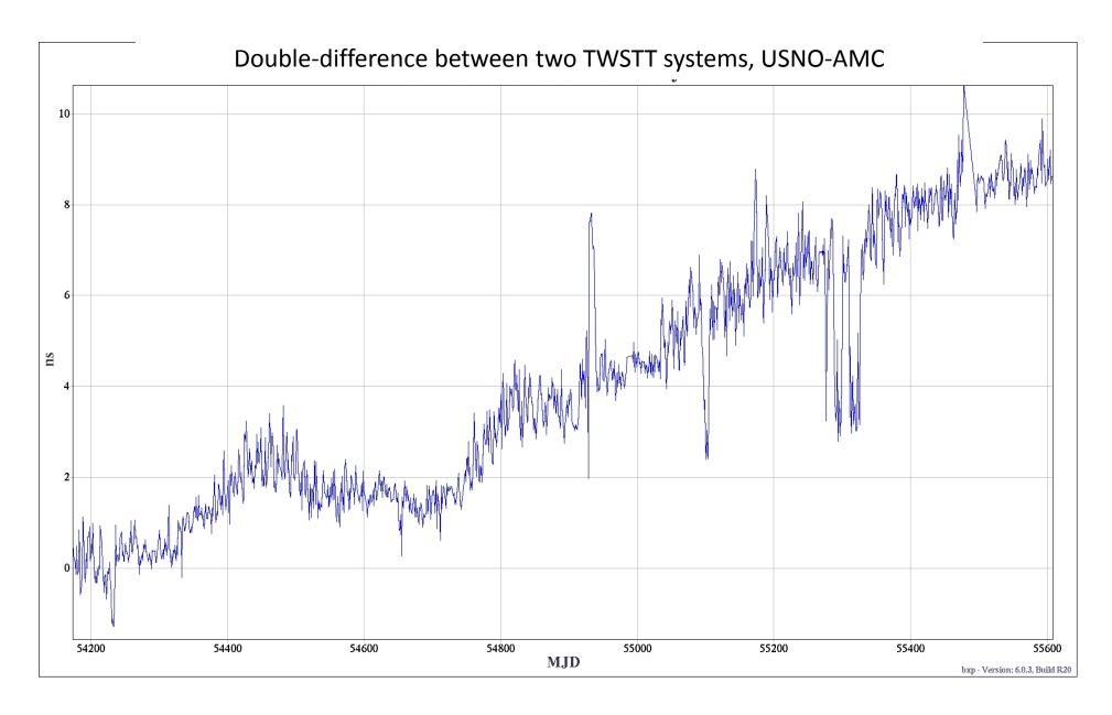
Delay shift could be due to electronics or fiber-optics feeding the TWSTT hardware
