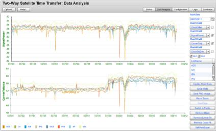
Quick plotting of signal power, frequency, carrier to noise, stddev, etc... for all links
