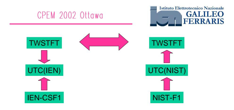
Synchronous measurements with Fountain and TWSTFT, rejects the noise of UTC(IEN)
