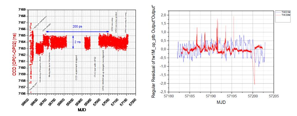
Analysis provided by Joseph Achkar, OP. The mean of OP01/OP02 common-clock difference remains a constant over 1.5 years. The mean of the OP/PTB 1MChip/s and 20MChip/s (broadband) TW double difference shows a good agreement over 20 days (using another technique to check the TW link variation).
