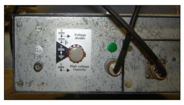
$\label{eq:photon} \begin{array}{l} \mbox{Photo 1.2-HV Capacitor-Switch position for AC voltage measurements.} \\ \mbox{Grounding of low voltage terminal of the $C_{13}$ capacitor.} \end{array}$
