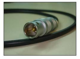
Photo 1.6 – Measuring Cable 1 – LEMO Connector FFA.3S.140.CTAC62 (to connect to the LV capacitor)
