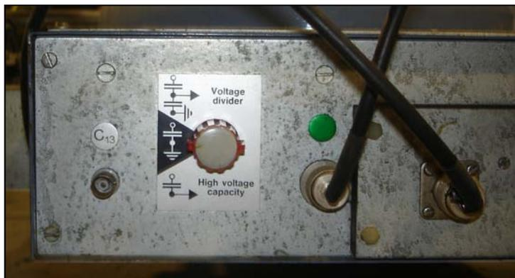
Photo 1.2 – HV Capacitor – Switch position for AC voltage measurements.
