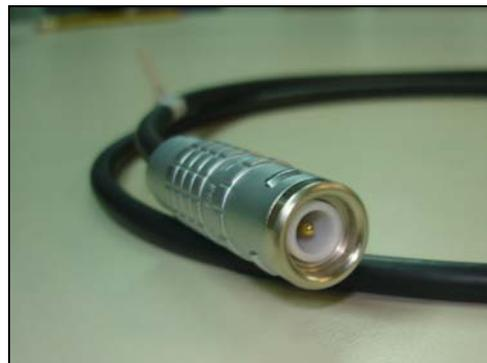
Photo 1.7 – Measuring Cable 1 – LEMO Connector FFA.2E.250.CTAC60 (to connect to the HV capacitor) Main capacitance  $C_{12}$  -
