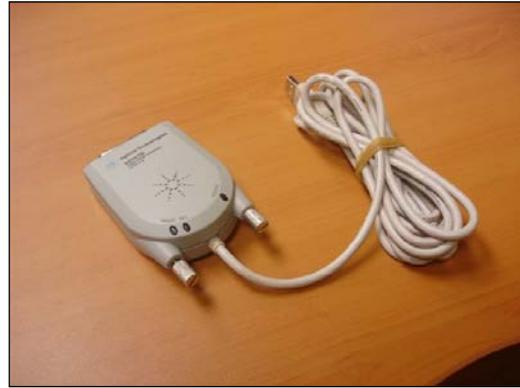
Photo 2.2 – Agilent USB/GPIB Card
