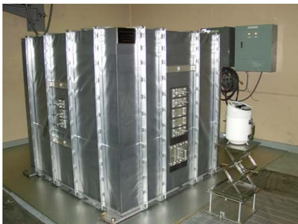
Fig. 5 Photograph of the graphite pile for thermal neutron calibration fields; Inside or outside of the pile is used for calibration.
