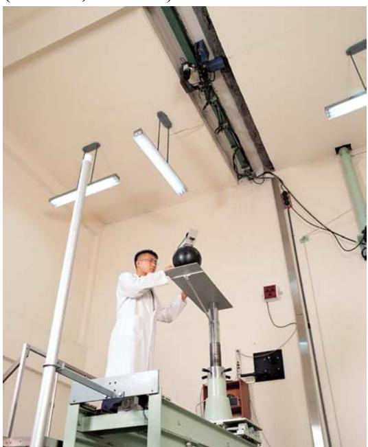
( $^{252}\text{Cf}$  with the neutron emission rate of  $\sim 10^8 \text{ n/s}$ ) can be controlled remotely. The moving arms for the calibration and test of the neutron detector can be moved about 2 m (the minimum distance from the source is  $\sim 20 \text{ cm}$ ).
