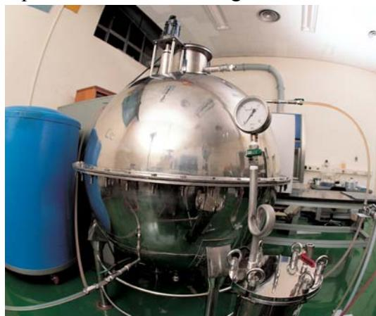
to the position of the gamma detector (NaI (Tl) crystal of  $1.5'' \times 1.5''$ ). The counting efficiency of the system is determined using the standard  $^{56}\text{Mn}$  radioisotope. The  $^{56}\text{Mn}$  radioisotopes are produced by the research reactor and the specific activity is determined by  $4\pi\beta-\gamma(\text{PPC})$  coincidence method, which is the KRISS primary standard.
