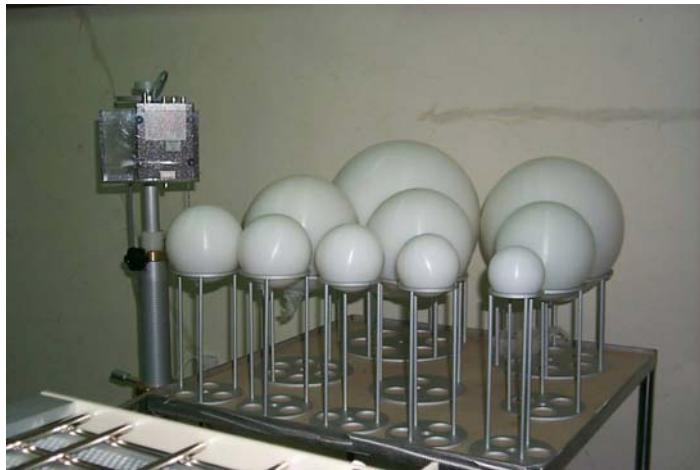
12" diameter and originally designed by PTB, Braunschweig. The response matrix is calculated by the small modification of original PTB BS's response matrix, considering the difference of the density and the size of the spheres. The normalization of the response matrix is determined by the measurement
