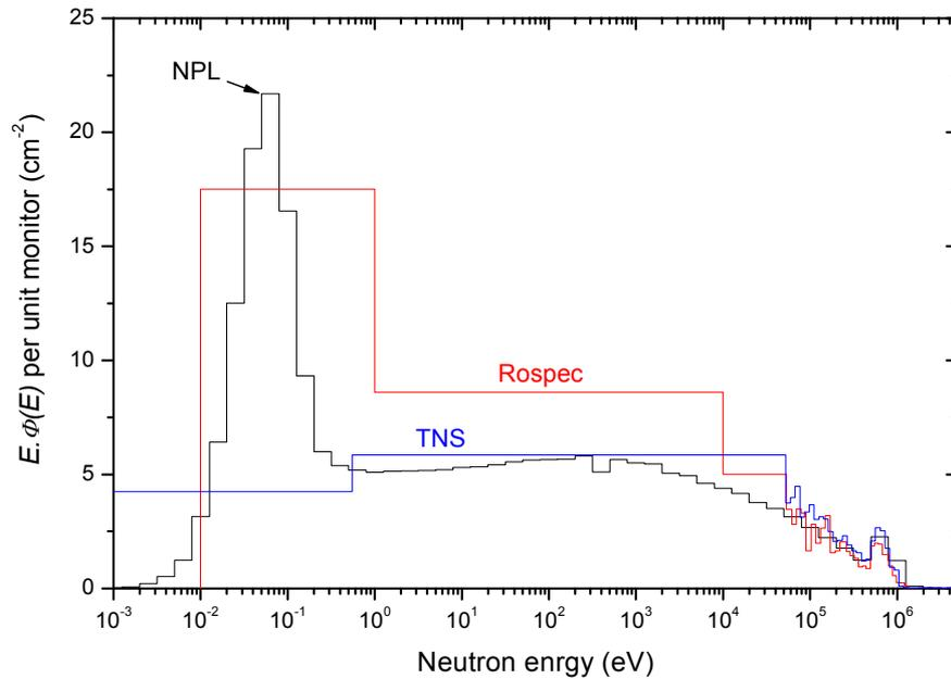
Figure 3. Results of spectrometric measurements with a ROSPEC and a Transportable Neutron Spectrometer (TNS) at the NPL simulated workplace field facility
