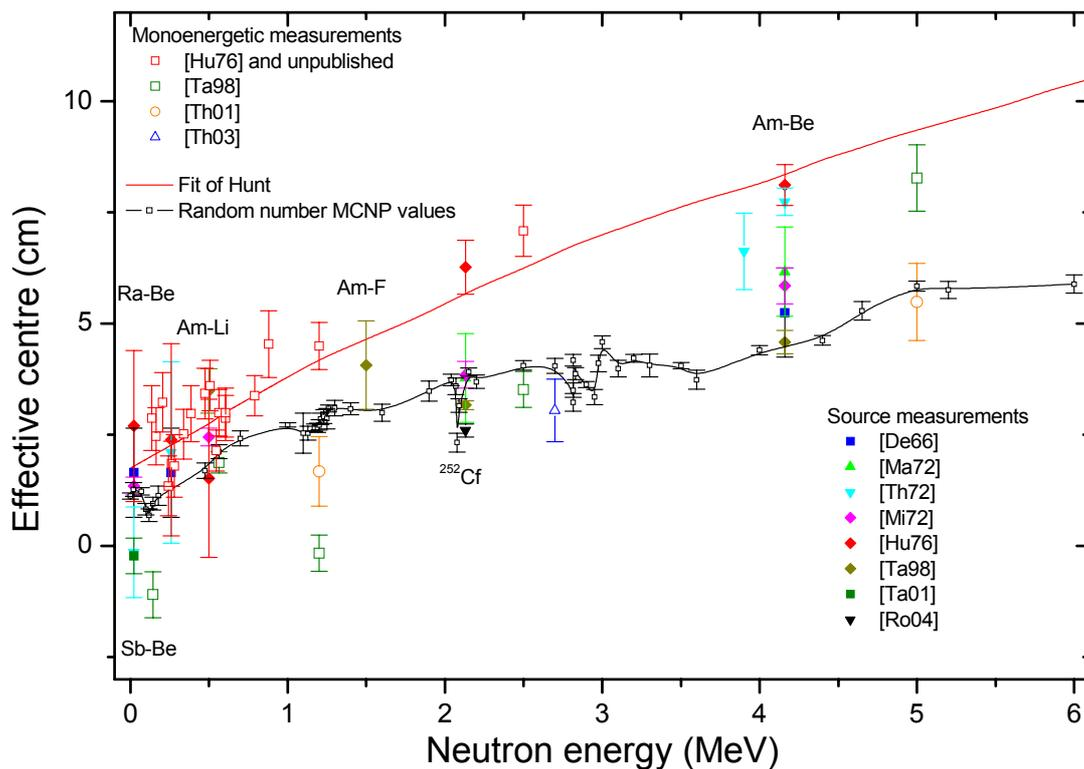
Figure 2. Effective center measurements for a De Pangher long counter compared with the empirical curve of Hunt and the calculations of Roberts et al<sup>4</sup>. All the monoenergetic data are from NPL, as are the source measurements of Hunt [Hu76], Tagziria [Ta01] and Roberts [Ro04].
