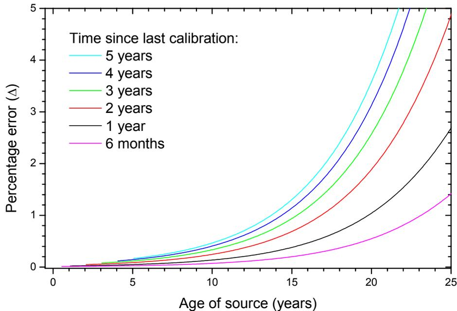
Figure 1. Percentage error in the neutron emission rate of a typical californium source when correcting for decay using the  $^{252}\text{Cf}$  decay constant.
