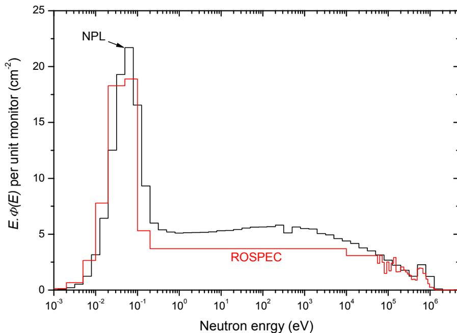
Figure 4. Revised analysis of ROSPEC measurements of simulated workplace field.
