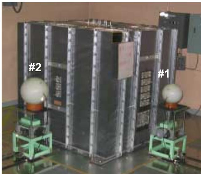
**Fig.1.** Photograph of the graphite pile for the thermal neutron calibration fields: There are two calibration points, #1 and #2, in front of different faces of the pile.
